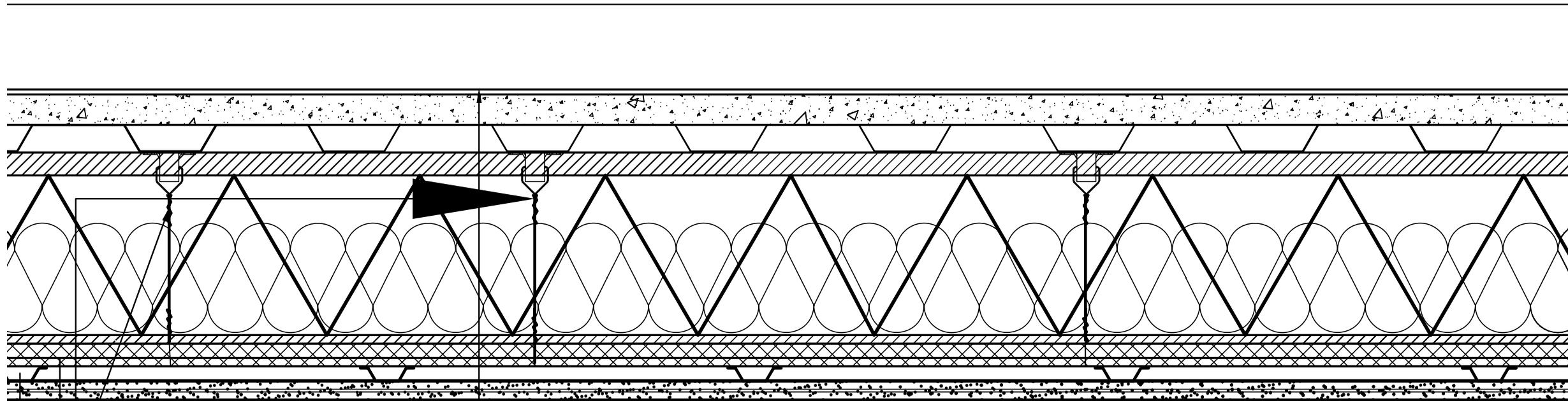
ESPACEMENT DES ANTI-VIBRATIONS 30" C/C
